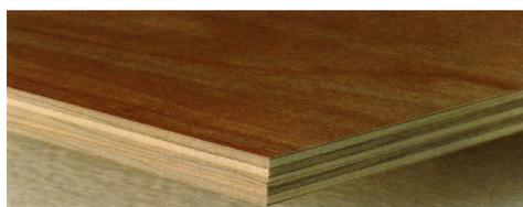
**Plywood** (Figure 4) is produced from three or more thinner sheets of veneer which are joined by an adhesive, with the wood grain of each layer running at right angles to the adjacent one. A distinction is made between lumber core *plywood* or *blockboard* (with a core of solid wood or veneers), *cellular board* (a core with a cellular structure) and *composite plywood* (with the core or certain layers made of a material other than solid wood or veneers).<sup>17</sup>
